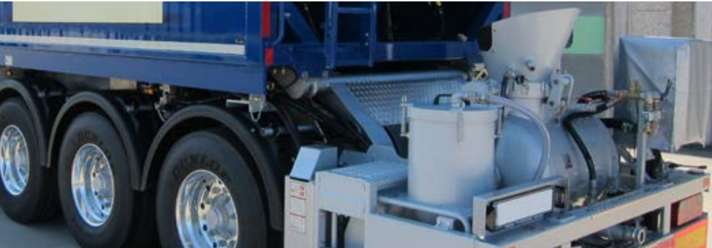
Semi-dry floor screed – mixing chamber with compressed-air conveyor (TransMix 5500)
